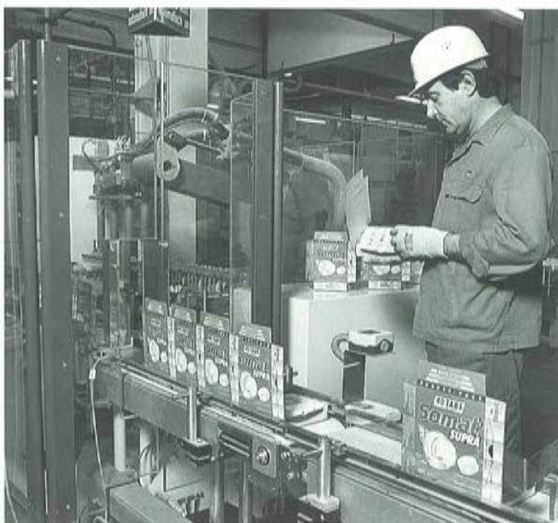
With the help of new machine technology on the production line, dishwasher cleaner tabs are inserted into the box layer by layer.
