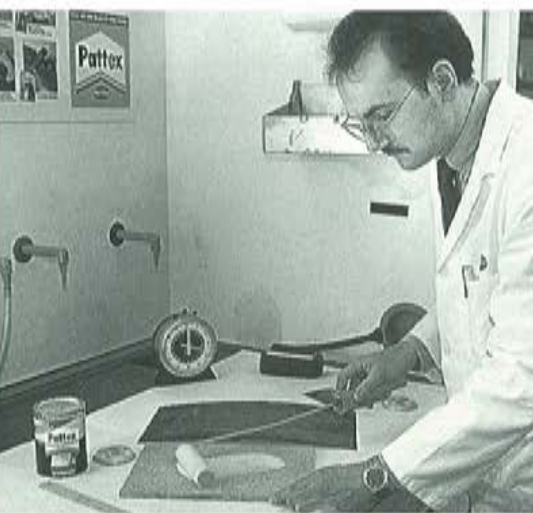
Testing the initial and final strength of the water-based contact adhesive.
