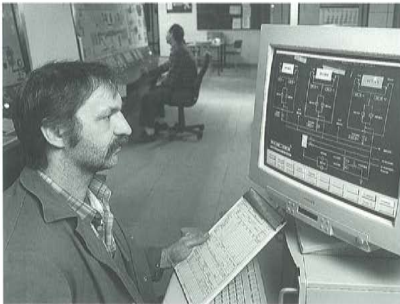
The emission values of the water glass factory are monitored at the control desk.
