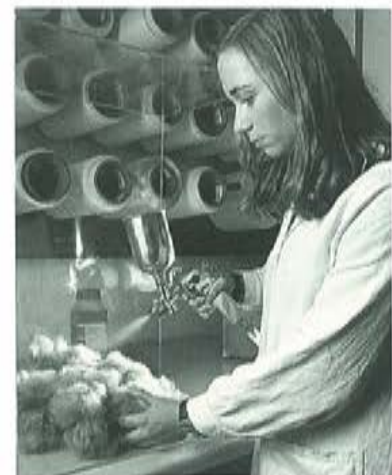
Washed wool is sprayed with combing lubricant in the laboratory.
