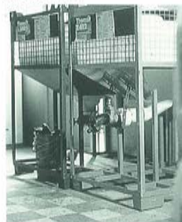
A filling point for emulsion primer. Workers transfer the product to handy canisters on site.
