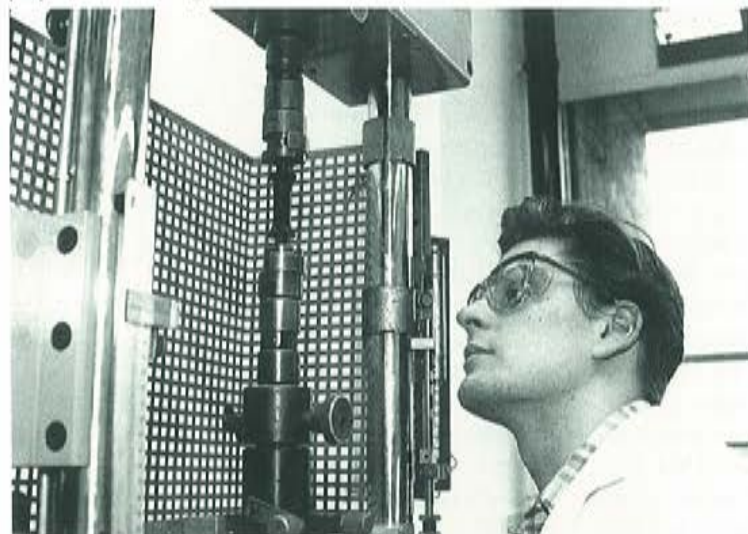
The tension test shows that aqueous bonding agents are on a par with solvent-based adhesives in terms of adhesive properties and strength.
