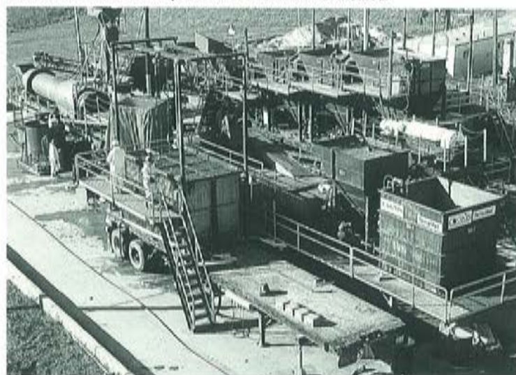
Plant with which soil containing lead was decontaminated in New Brighton, USA. The concentration of heavy metals was reduced from 8.6 to 0.02 percent with the TerraMet method.
