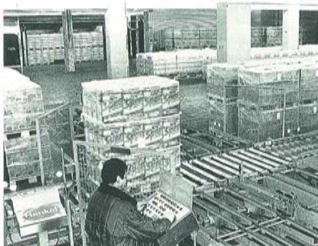
Modern computer technology controls the dispatch of the various detergent pallets which, bar-coded, automatically roll onto the right loading ramp.
