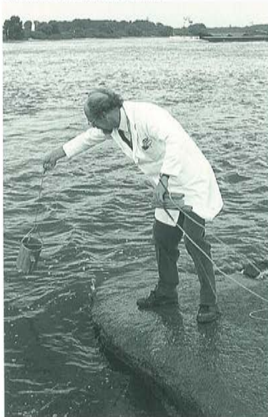
Samples of water are taken annually at 140 sites on the Rhine and its major tributaries and analyzed for chemical pollution.
