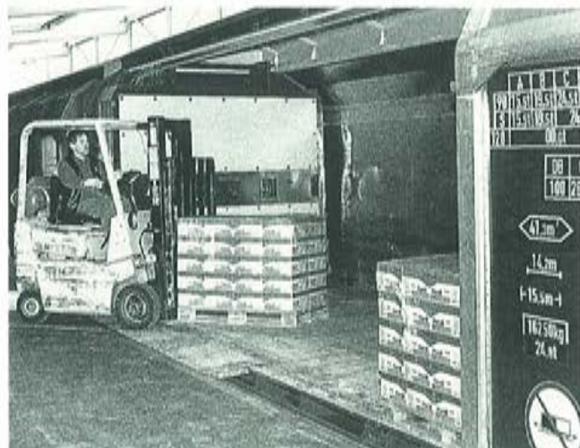
In a non-stop process, the detergents and cleaning agents are forklifted from the production line directly into freight cars (here at the Düsseldorf parent plant).
