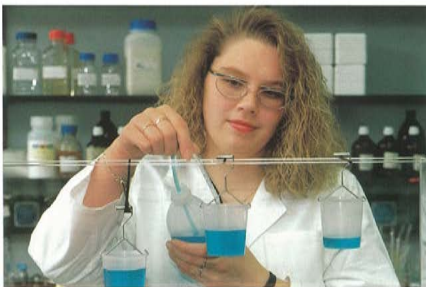
A hair strand treated with chitosan is tested for its bending strength by suspending a beaker from it. The more water that can be added to the cup, the greater the strength imparted by the chitosan solution.
