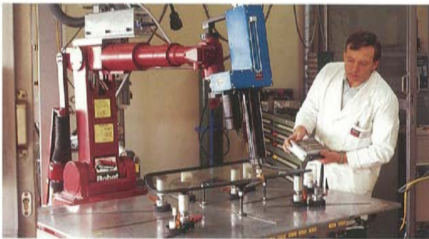
Adhesives for direct glazing of windshields: testing an applicator robot at Henkel Teroson, Heidelberg.
