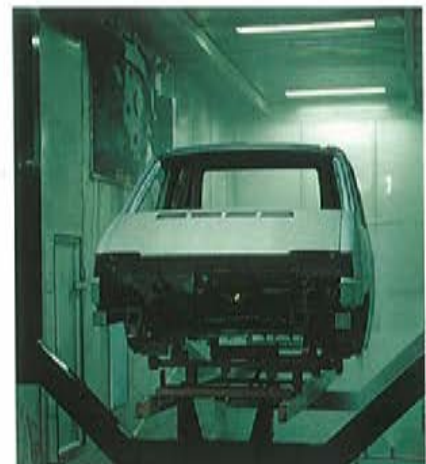
Autobody pretreatment: the phosphating step is important for the adhesion of the subsequently applied paint, and as an anticorrosion measure.
