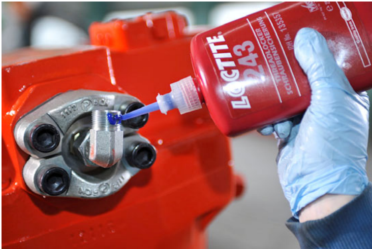
This threaded fitting has to resist up to 350 bar oil pressure.
