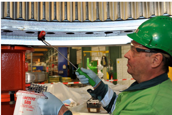
At the montage different gear units are bonded and bolted together.
