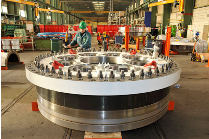
Completed main drive is waiting for the assembly into the machine.
