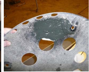
Plastic repair on the hub cap of Japanese Hino Ranger - Pro FT truck no. 507
