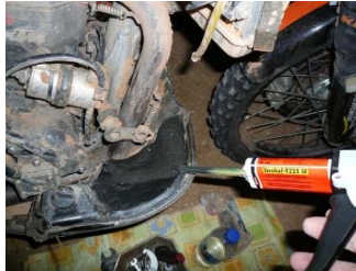
Terokal 9225 SF was used to repair this water tank
