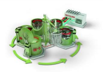
The fully automatic Loctite impregnation process serve to reliably seal all forms of porosity in alloy castings, sintered metals, ferrites, ceramics and composite materials.
