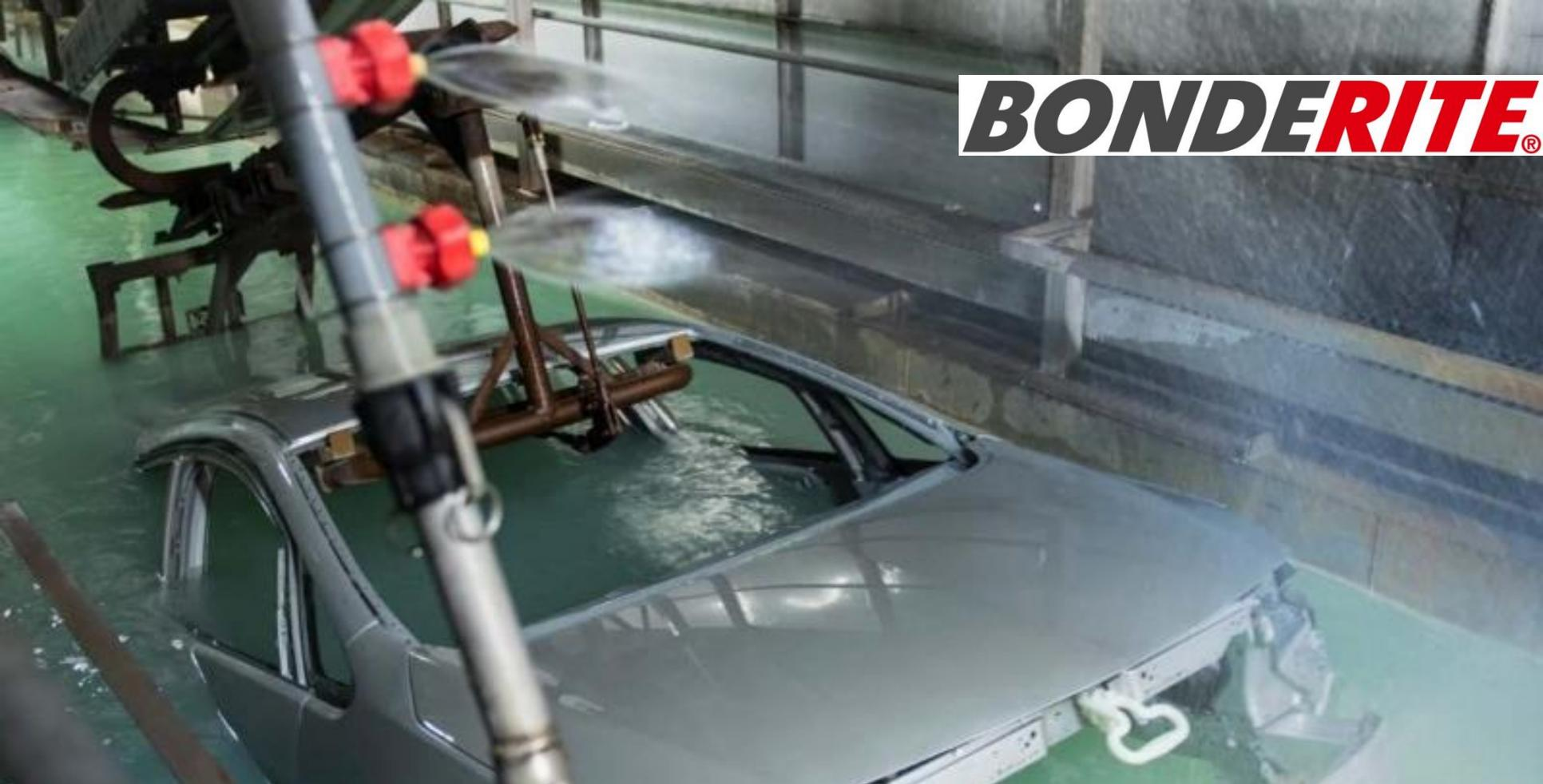
A close-up view of a car body in a paint booth. A high-pressure water spray is directed at the car's surface from a nozzle. The spray is creating a mist of water droplets. The car body is metallic and appears to be in the process of being cleaned or prepared for painting. The background shows the industrial structure of the paint booth.
