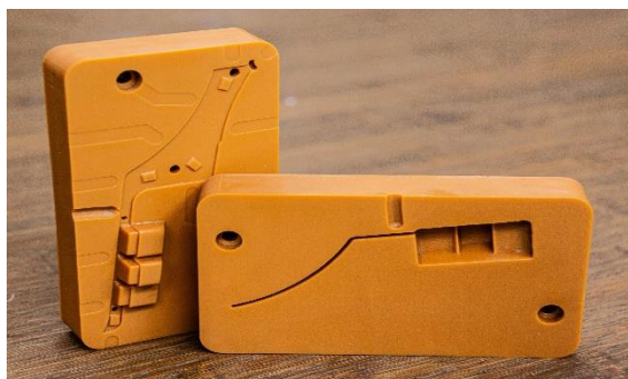
A 3D printed tool by Fortify which is used to mold an automotive part
