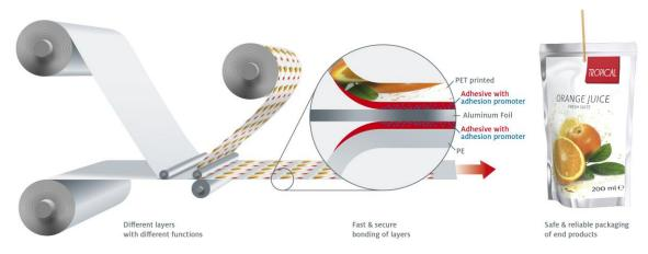
The architecture of multi-layer packaging is highly dependent on high-performance adhesives and suiting adhesion promoters, which enable a lasting and secure bond of materials
