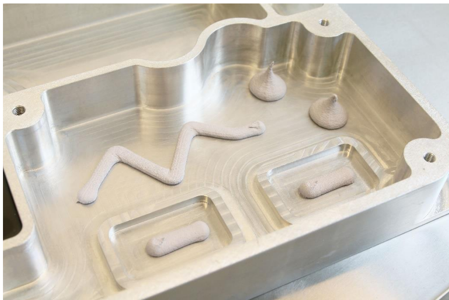
Result after a dispense trial of the Bergquist TGF 7000 with Bdtronic. (Photo credit: Bdtronic)
