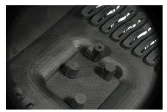
Detailed view of the 3D printed electronic housing part with ventilation slits and openings for cables and electronics
