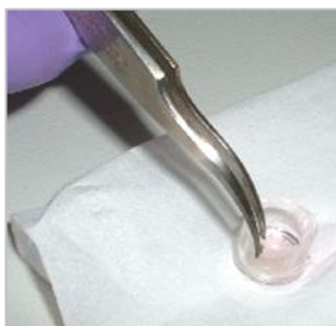
Figure 4: Blotting and drying of the surface
