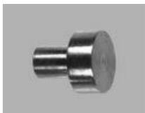
**Figure 3:** Stainless steel aid, used for applications with waxy test substances
