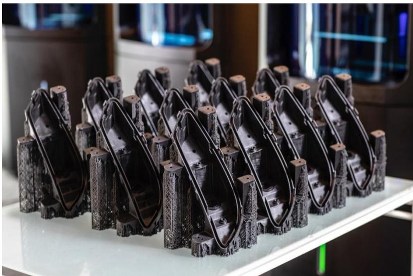
High accuracy parts printed with xPRO410 (fast print photopolymer) on Nexa3D's NXE400 printer.
