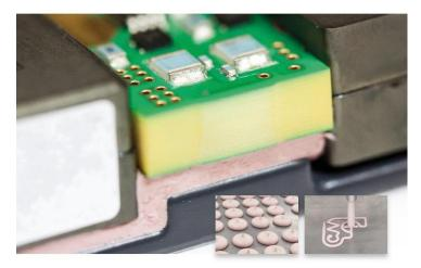
Bergquist Gap Filler TGF 4500CVO is a liquid, gap filling thermal interface material that accelerates dispensing, reduces contamination risk and improves reliability.
