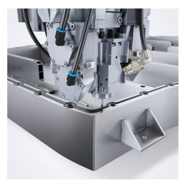
Precisely contoured double seal application on the battery housing with polyurethane sealing foam Sonderhoff Fermapor K31.
