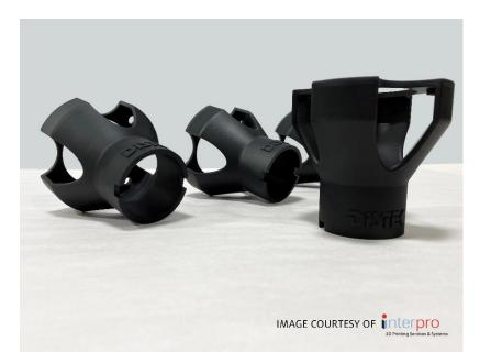
Adaptors for medical bio-reactor equipment developed and printed by InterPRO and Henkel with Loctite 3843 black.
