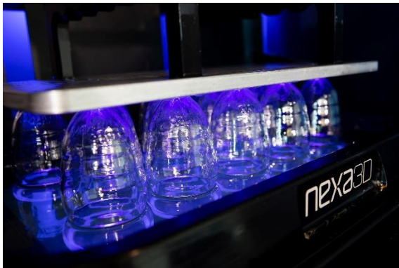
3D printed bottles using the new xPP405-Clear material: the excellent clarity enables new applications for end-use packaging or bottling for example.
