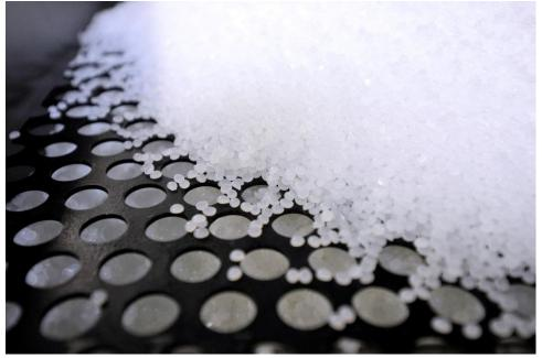
The new high-performance hot melt adhesive range includes two grades with up to 98% bio-based content and provides a way to optimize the carbon footprint of end products and packaging.
