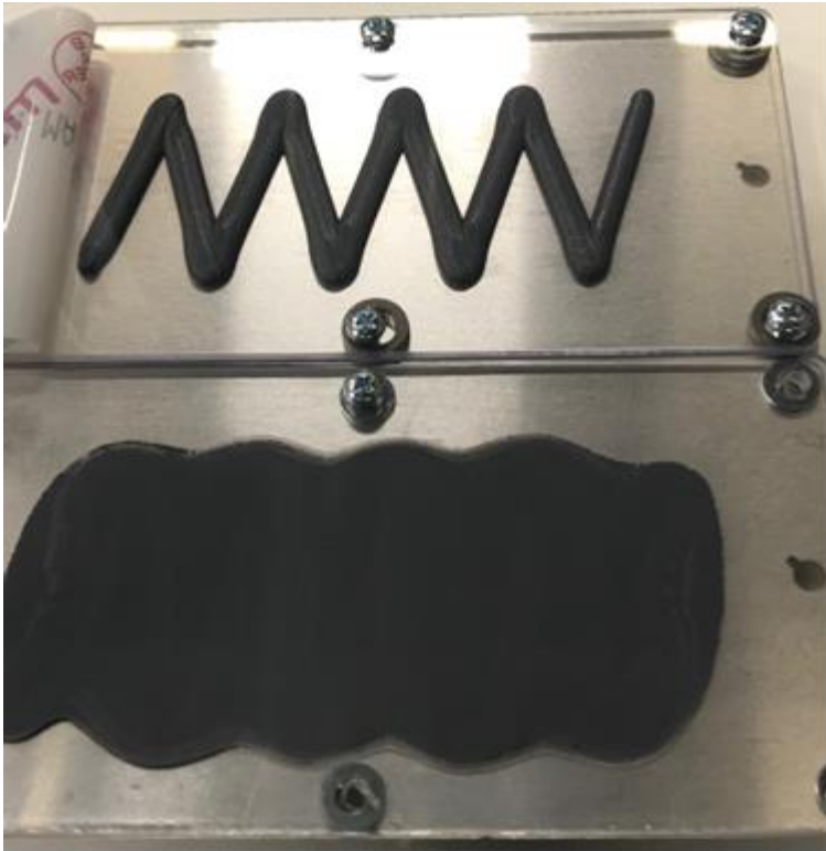
Bergquist Gap Filler TGF 3010 APS shows exceptional results in material quality and ease of removal after accelerated stress testing carried out in Henkel laboratories
