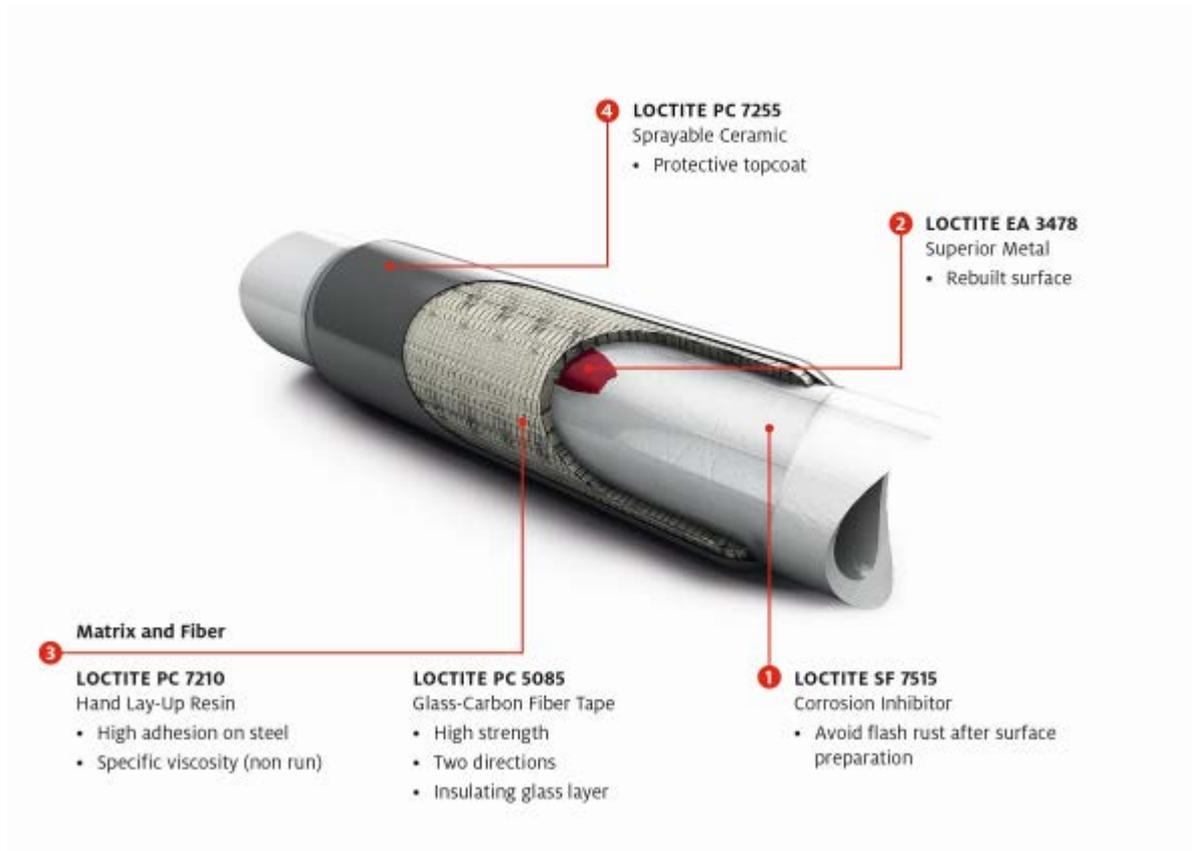
The Loctite Composite Repair System repairs and protects steel pipes constructed to withstand high pressure, high temperatures and chemicals.
