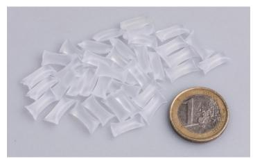
The small, non-sticky mini pillows of adhesive can freely flow to allow auto-feeding into the melters.
