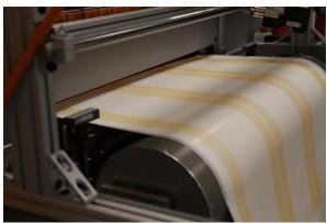
The automated system print the feed spacer directly on to the flat sheet web. In this image, three 1812 patterns are printed side by side.
