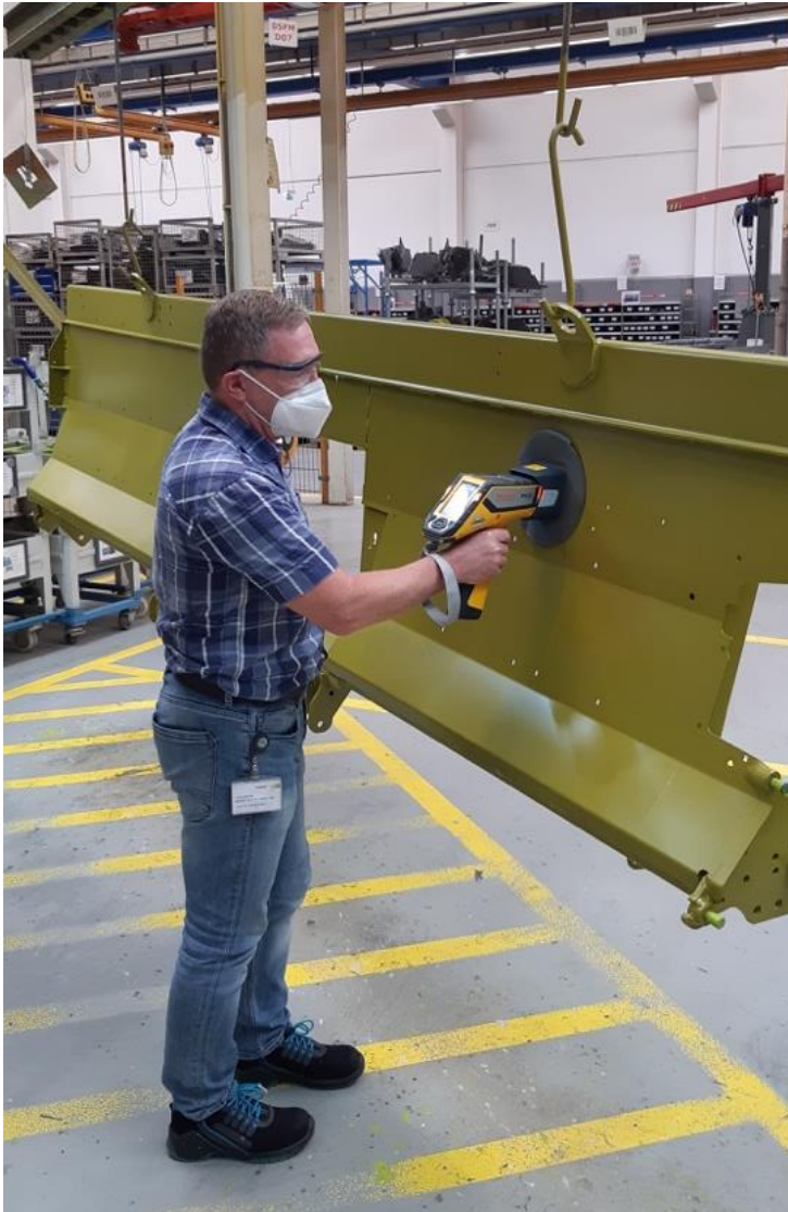
Measuring the coating weight of the ZnPO4 layer through the e-coat at Claas Bad-Saulgau.
