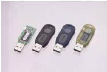
With the hotmelt adhesives under the Technomelt brand, it is possible not only to bond surfaces but also to provide protective encapsulation even for small and delicate electronic components.
