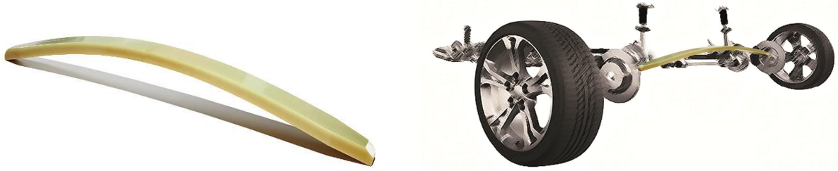
Photos 1 and 2: Composite leaf springs as manufactured (left) and as installed (right).
