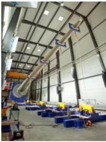
The adhesive bonded joints performed well during the endurance test under extremely heavy loads. The IWES tested the 40-meter-long rotor blade in accordance with the IEC 61400-23 standard, which is used to examine nominal load capacity and fatigue damage during static and dynamic tests.
