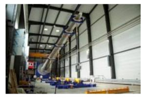
An ENERCON rotor blade manufactured using Macroplast UK 1340 underwent an endurance test lasting around four months at the Fraunhofer Institute for Wind Energy and Energy System
