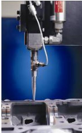
Offering tailored process know-how, Henkel facilitates the simple and efficient application of its liquid gasketing compounds.
