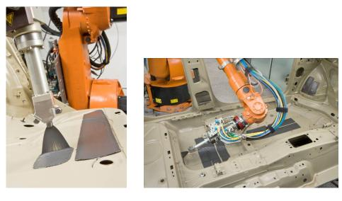
Teroson RB 8275, a liquid applied sound deadener (LASD), significantly reduces the solid-borne noise generated by the engine and the wheels during driving.
