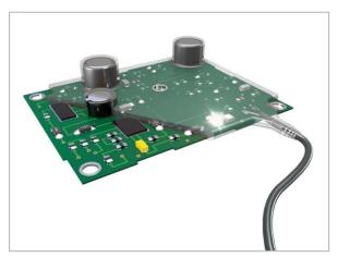
Low pressure molding is used to encapsulate PCBs used in medical diagnostic and monitoring devices to protect them from moisture, temperature and chemicals.
