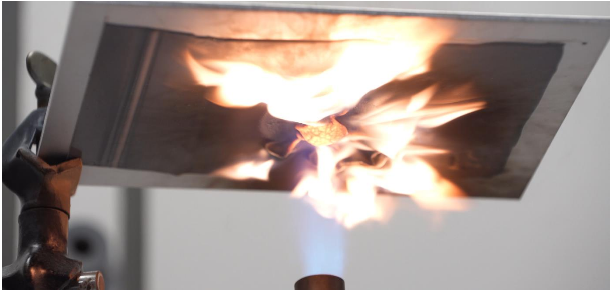
Image captured live during an open flame test; one of the testing methodologies that Henkel uses to test the performance of the fire protective coating products.
