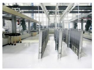
Henkel Adhesive Technologies offers various solutions for the pre-treatment of aluminum, for example in the form of battery housing cases.
