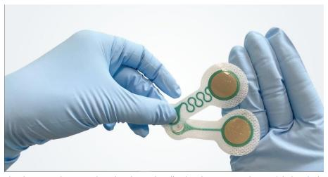
The demo patches contain a dry electrode adhesive that ensures the crucial electrical contact with the skin.
