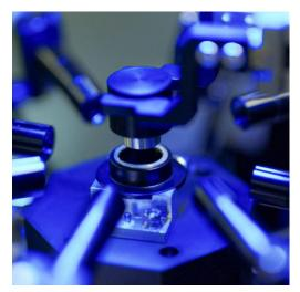
Using a unique UV cationic thermal dual cure epoxy, Loctite Ablestik NCA 3218 offers an ideal solution for lens bonding in ADAS sensors.
