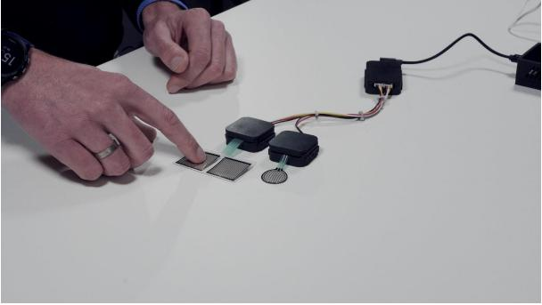
The Sensor INKxperience Kit offers IOT engineers the possibility to explore the potentials of printed electronics for the development of new sensor solutions.
