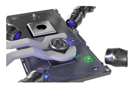
Active alignment, a state-of-the-art assembly method, used to manufacture high-quality camera modules, is the foundation for the safety-critical functionality of advanced driver assistance systems (ADAS) used in today's automobiles.
