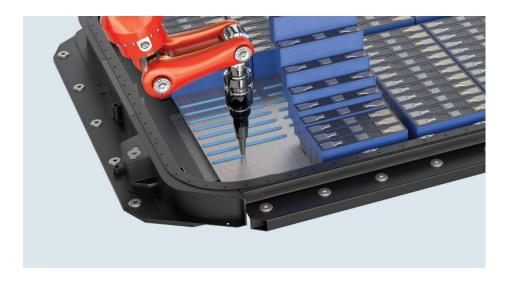
Illustrative image showing the application of Loctite TLB 9300 APSi between battery cells and the cooling system.
