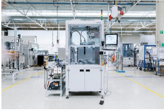
Semi-automatic machine from Henkel's dispense partner, bdtronic, for manual loading for various dispensing applications.
