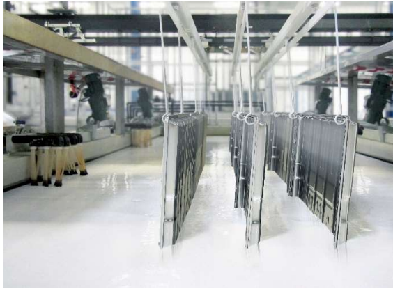
Aluminum battery housing during the metal pretreatment process
