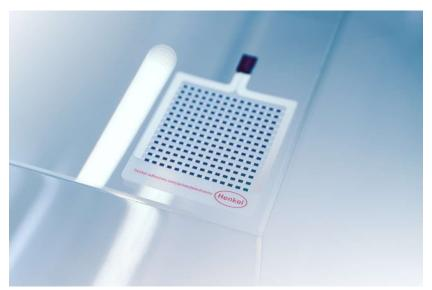
Henkel highlights innovation portfolio for end-use printed electronics applications at LOPEC 2024 with a focus on printed self-regulation PTC heaters.
