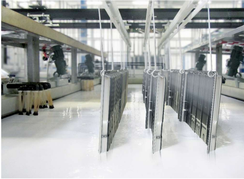
Chromium-free etch passivation process for light metal battery housings
