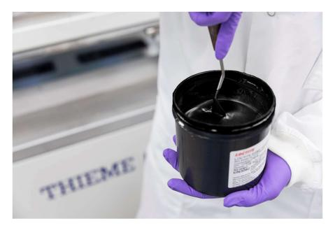
Henkel is providing its expertise in the development of Positive Temperature Coefficient (PTC) inks ensuring optimal electrical performance of the self-regulating heating elements.
