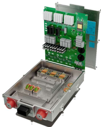
Graphic illustration of an integrated power conversion unit featuring thermal potting applications.
