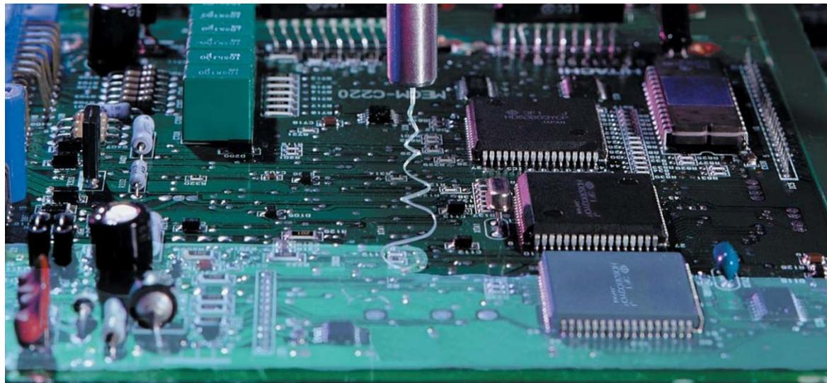
Conformal coatings are applied to PCBs and components to help protect them against moisture, dust, chemicals, and other environmental conditions.
