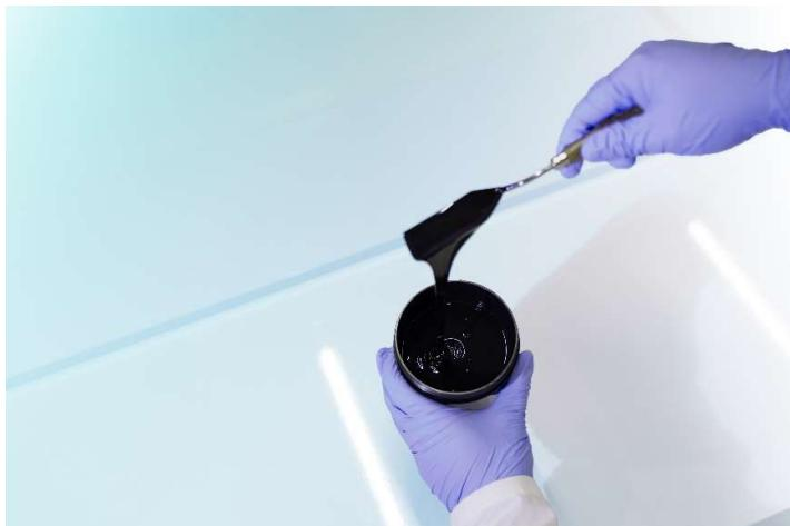
In combination with silver and dielectric inks, Henkel's Positive Temperature Coefficient (PTC) technology enables the screen printing of self-regulating foil heaters.
