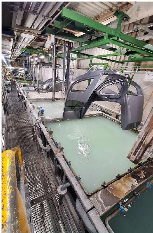
Bonderite C-AD 20202 is a new low-temperature surfactant for industrial dip degreasing that cleans reliably at temperatures as low as 35 to 40 degrees Celsius.
