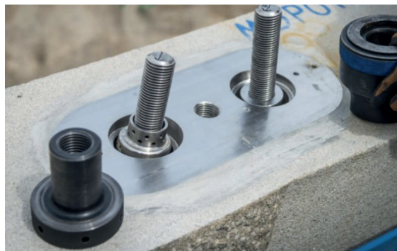
Figure 5. Machined stone pieces and steel elements designed for structural integration prior to adhesive application.
