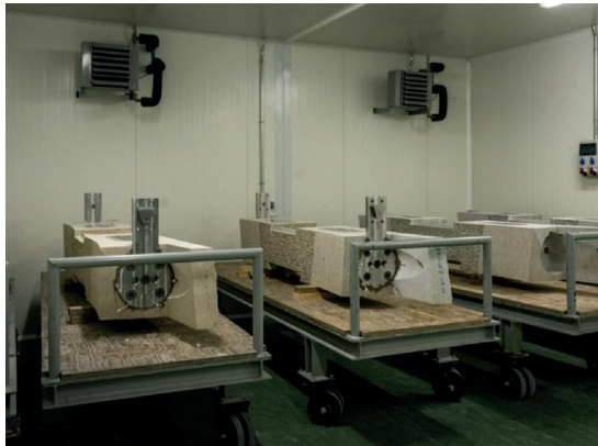
Figure 8. Image of the curing area where the bonded components, stone and steel, are kept at a stable and controlled temperature for 24 hours thanks to the adhesive.
