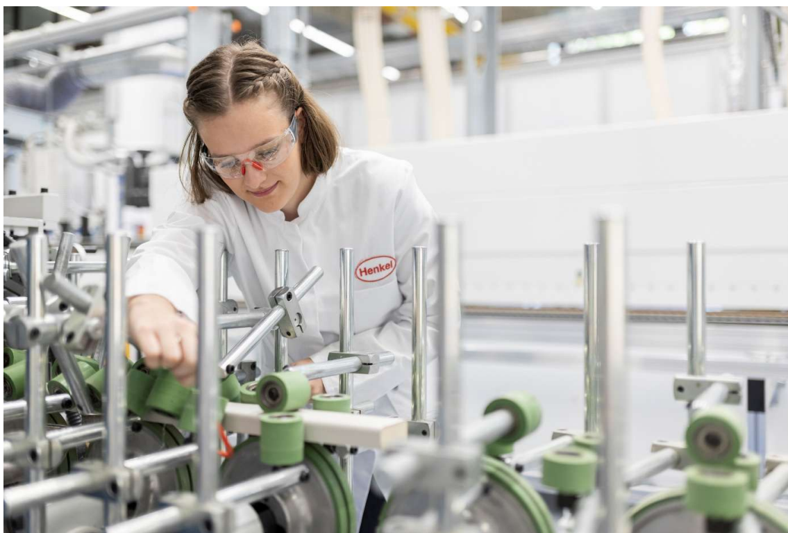
A Henkel technician sets up an edge banding machine for kitchen furniture production, where steam, temperature fluctuations and constant humidity put every adhesive bond to the test.
