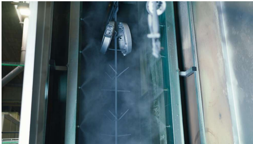
APNR technology sprays the adhesion promoter directly onto the metal surface at the end of the line, eliminating the need for a subsequent rinse stage.
