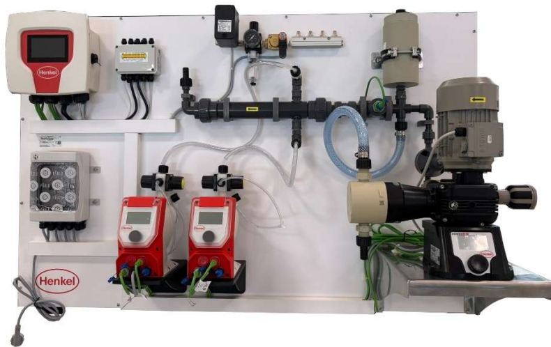
Henkel's new APNR 2.0 equipment generation: The EcoFlex control unit supports precise and repeatable application of the adhesion promoter.
