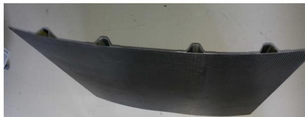
Hat-stiffened curved panel demonstrator produced using BZ 9130 resin.
